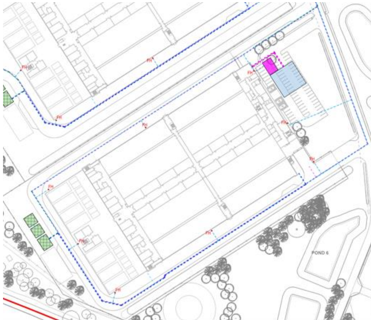
Figure 3-20. Extract from Watermain Layout indicating arrangement at typical data hall.
